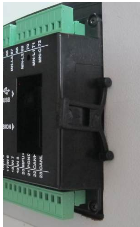
Installation of self retaining type bracket
